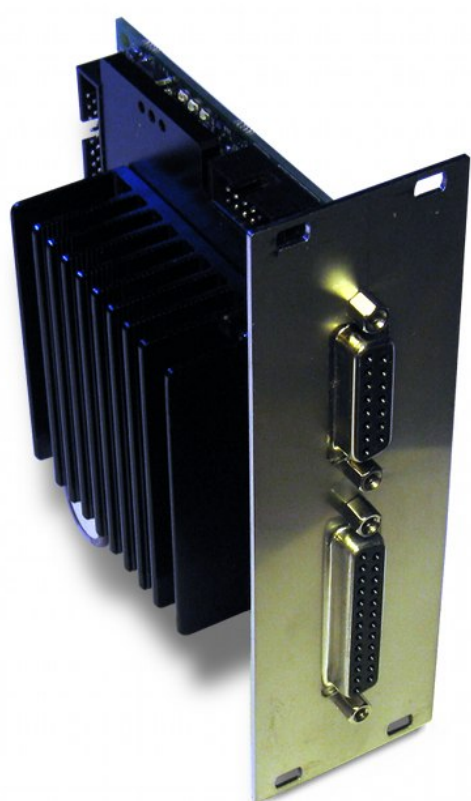
VSD-E fitted with additional heat sink and installation panel
