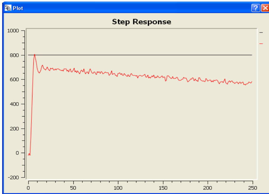
Figure 7: Current response test plot, P-gain tuning
